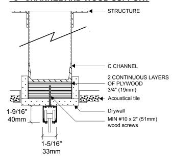
SUPPORT BUILT BY GENERAL CONTRACTOR MINIMUM WEIGHT CAPACITY OF 3 lb / sq. ft (15 kg / sq.m) OF GRILLE
