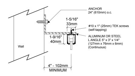
SUPPORT BUILT BY GENERAL CONTRACTOR MINIMUM WEIGHT CAPACITY OF 3 lb / sq. ft (15 kg / sq.m) OF GRILLE
