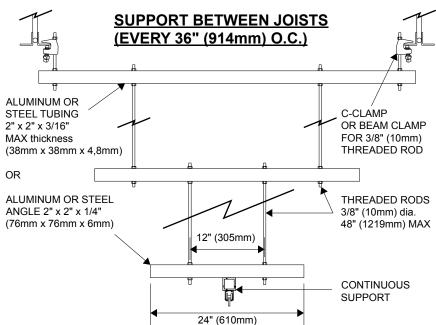
SUPPORT BUILT BY GENERAL CONTRACTOR MINIMUM WEIGHT CAPACITY OF 3 lb / sq. ft (15 kg / sq.m) OF GRILLE
