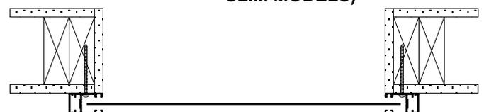
All wood support must be continuous and attached to building structure
